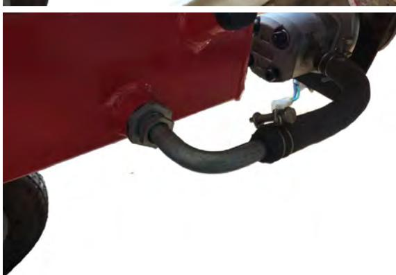
After completion, plug in the oil pipe again and tighten the steel hoop by spanner.
