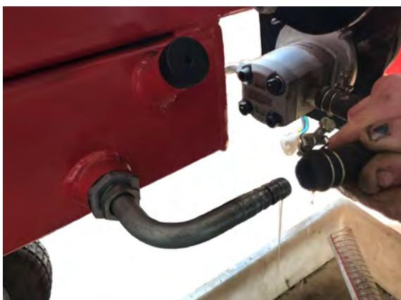
Place the log splitter over a container with the capacity of at least 4 liters. Pull out the oil pipe to drain oil.
