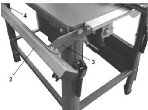
2. Using a spacer plate (A), fit the complete guide tube onto the left side of the table plate between table and front support (3).
