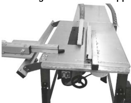
6. Setting the sliding table guide: The ball bearing guide can be set by releasing bolt A. If the table is too easy-running, release bolt A and displace the ball bearing upward. Then retighten the bolt. If the table is too tight, release bolt A and displace the ball bearing downward. Then retighten the bolt. Make sure that the guide rail is always clean.
