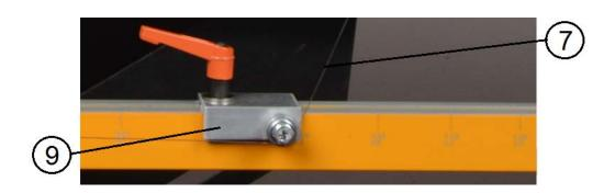
By means of the spring (10) and positioning of the end block (8), adjust the wire (7) to the desired tension.
