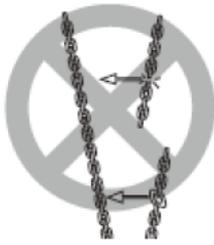
1. NEVER use a twisted, kinked, damaged or stretched load chain.
