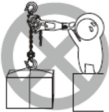
4. NEVER lift up load beyond the rated capacity of the hoist.
