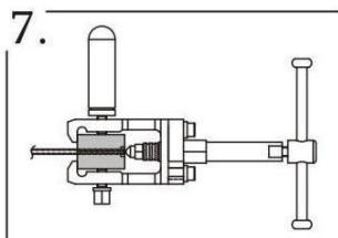
Twist the S-slider in place and use the T-bar again.
