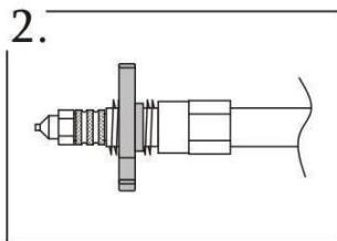
Insert desired adapter and screw the S-slider to approximately half way up the thread.
