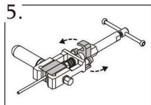
Return the T-bar and disengage the S-slider.
