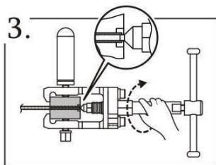
Twist the S-slider in place and turn the arm until the adapter head enters the pipe.
