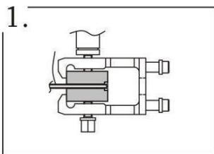
Place the pipe end flush with the die block edge.
