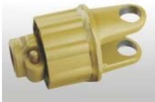
3. SHEAR BOLT TORQUE LIMITER: It stops the transmission of power when the torque exceeds the calibration value. Replace the bolt with a bolt that has same dimensions and resistance class. Grease once every season and after storing.
