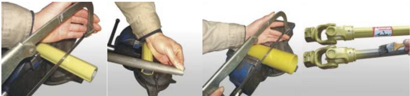
1. Remove the guards. Hold the half-shafts next to each other in the shortest working position and mark them. The overlap is proper if the shaft could be 5 cm in the shortest position. The two tubes should not touch the end of the PTO shaft, but you should not shorten the shaft too much. Shorten inner and outer guard tubes equally.
