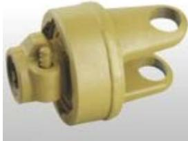
2. RATCHET CLUTCH TORQUE LIMITER: It stops the transmission of power when the torque exceeds the calibration value. Disengage the drive immediately when you hear the release of the ratchet teeth. Grease every 50 hours and after every period of inactivity.
