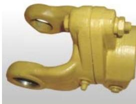
4. FRICITION-TYPE TORQUE LIMITER: Limits torque transmission to the calibration value. Do not change spring compression, as this will modify the device settings. The torque setting is adjusted by increasing or decreasing the height of the springs. Tighten/loosen the eight nuts by  $\frac{1}{4}$  of a turn and check for correct operation. Repeat the procedure if necessary. Avoid excessive tightening of the bolts in order to avoid damage to the implement, tractor or driveline. Do not grease.
