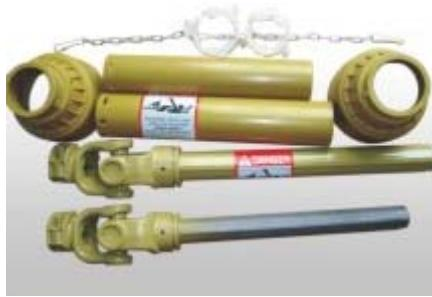
1. FREEWHEEL: Eliminates power returns from the machine to the tractor during the deceleration or stop phases of the power take-off. Keep away from the appliance until all parts have come to a complete stop. Grease every 50 hours and after every period of inactivity.
